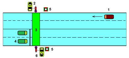
Fig. 6. Sound measurement at a pedestrian crossing in urban traffic: 1 – test automobile; 2, 6 – measurement positions; 3 – pedestrian crossing; 4 – vehicles generating background noise; 5 – traffic light
