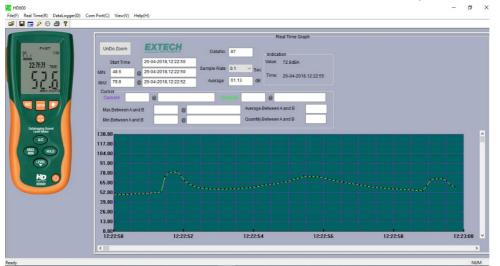
Fig. 3. Screenshot of the application window for the sound level meter
