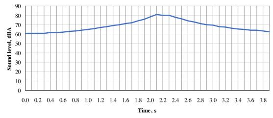
Fig. 8. Change in the noise level for the Renault Clio EV travelling at a speed of 50 kmh<sup>-1</sup>
