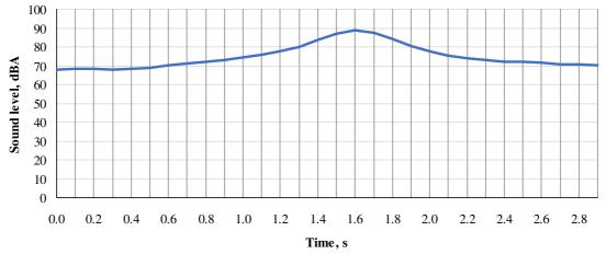
Fig. 9. Change in the noise level for the Renault Clio EV travelling at a speed of 90 kmh<sup>-1</sup>
